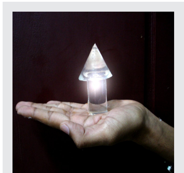
Figure 1: Optical component made of organogels. A cylinder and a cone made of organogels are combined to produce this optical tower, which can be held safely in the palm of a hand, and which remains stable for months.
