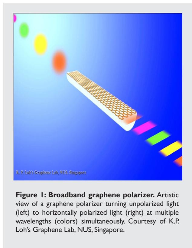
**Figure 1: Broadband graphene polarizer.** Artistic view of a graphene polarizer turning unpolarized light (left) to horizontally polarized light (right) at multiple wavelengths (colors) simultaneously. Courtesy of K.P. Loh's Graphene Lab, NUS, Singapore.
