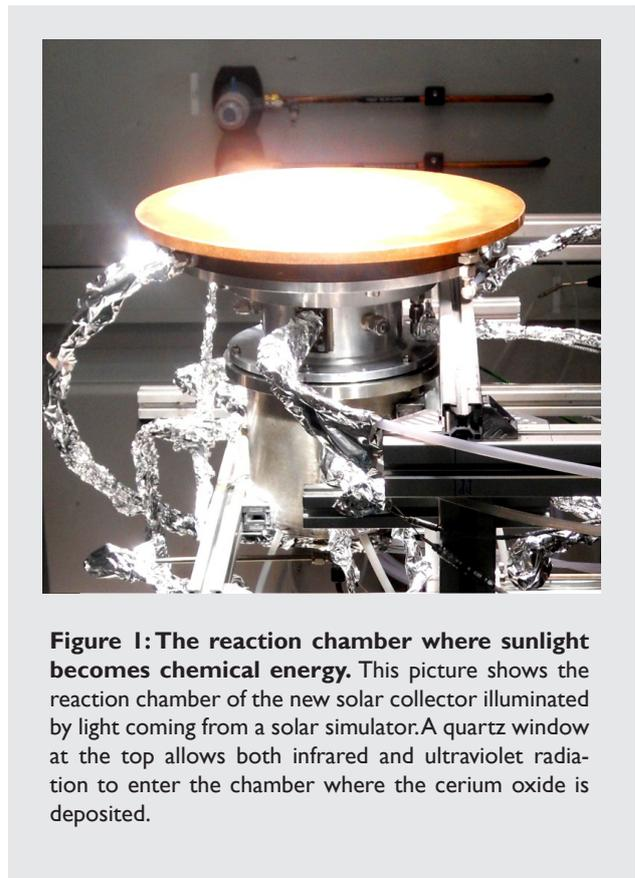
**Figure 1: The reaction chamber where sunlight becomes chemical energy.** This picture shows the reaction chamber of the new solar collector illuminated by light coming from a solar simulator. A quartz window at the top allows both infrared and ultraviolet radiation to enter the chamber where the cerium oxide is deposited.
