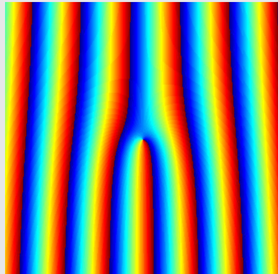
Figure 2: The pitch-fork hologram. The pitch-fork hologram, which has been traditionally used to generate optical vortices, can now also be used to generate electron vortices. The singular point at the centre is the main reason for the production of the vortex, and it also gives the hologram its name.
