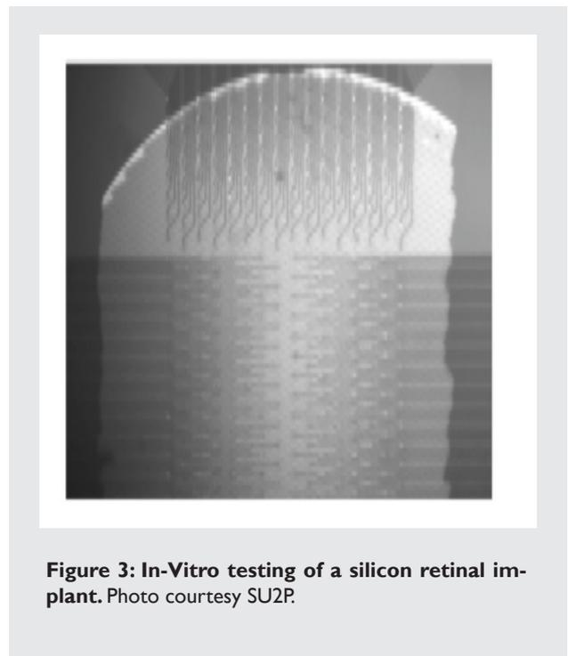
**Figure 3: In-Vitro testing of a silicon retinal implant.** Photo courtesy SU2P.
