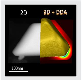
**Figure 1: 3D tomography of a nanoparticle.** The 3D shape of a nanoparticle can be reconstructed from many 2D SEM images of the same. Once the 3D morphology of the nanoparticle is known, its optical response can be calculated with the algorithm developed by the researchers at the National University of Córdoba.
